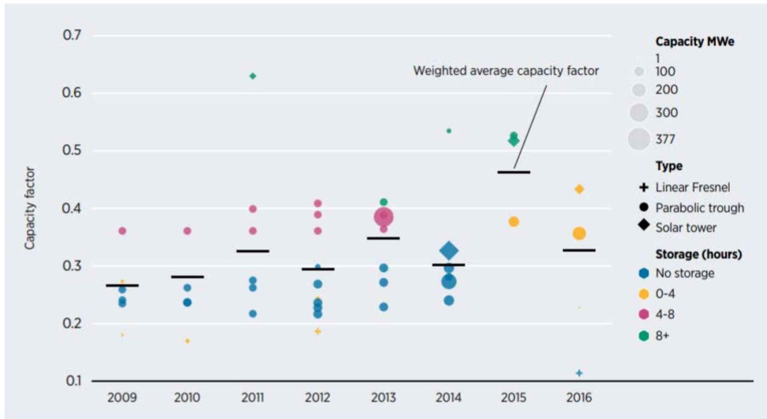
Figure 4.7 Capacity factor trends for CSP plants, 2009-2016
