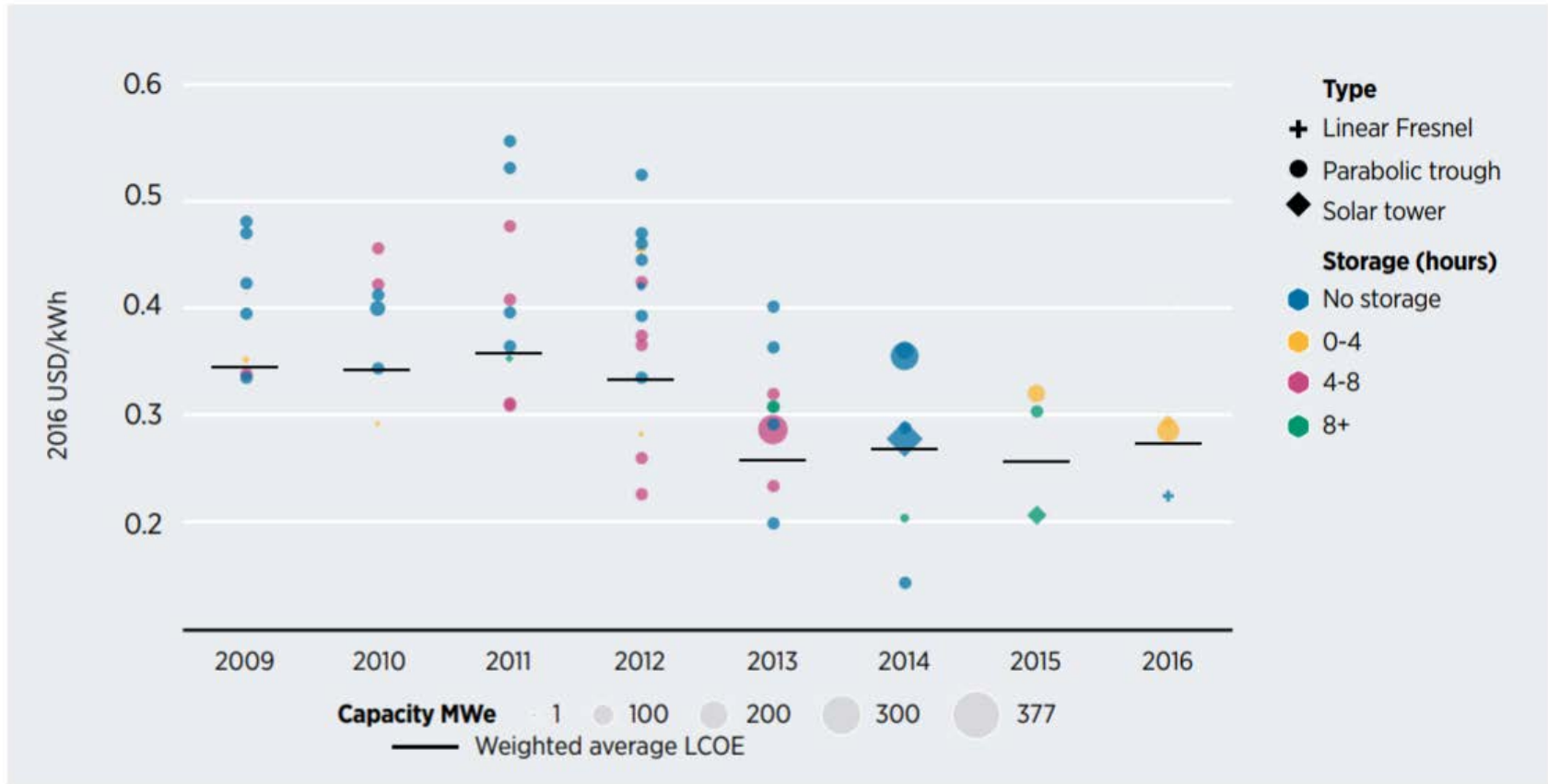
Figure 4.9 The levelised cost of electricity for CSP projects, 2009-2016
