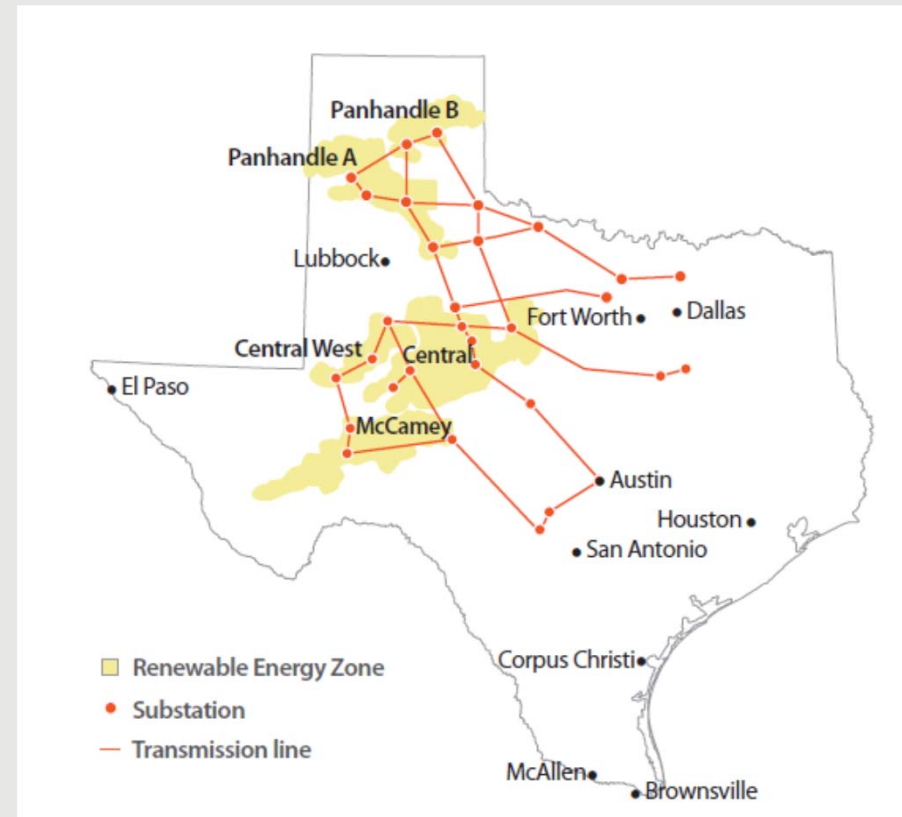
REZs and new transmission infrastructure to access zones - Texas Competitive Renewable Energy Zones (CREZ) (Hurlbut, Chernyakhovskiy, and Cochran 2016)
